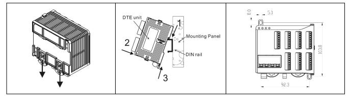
Connect maximum 7 DTC2000 or DTC2001 controllers to DTE by using DIN rail.
